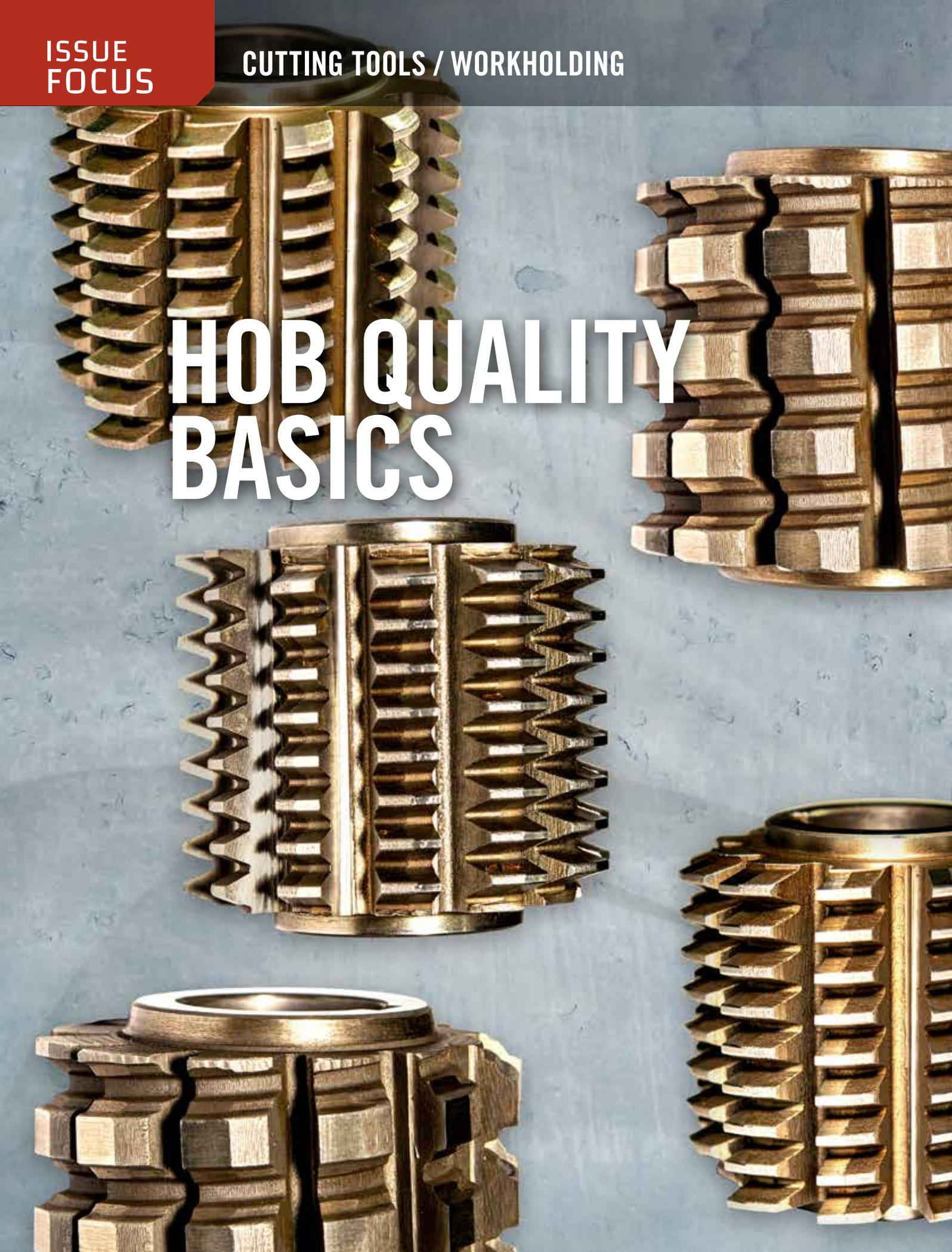
The image features five distinct metal hob cutters, which are cylindrical tools with multiple cutting edges. They are arranged in a circular pattern around the central text. The cutters vary in their tooth profiles, including standard double-flute, triple-flute, and more complex multi-fluted designs. The background is a light blue, textured surface, possibly a wall or a large metal plate. The lighting is dramatic, highlighting the metallic sheen and the sharp edges of the teeth.
