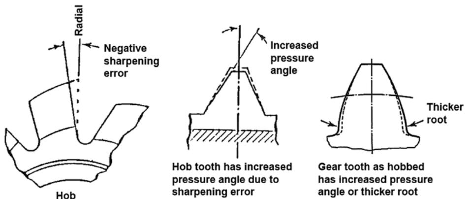
Figure 5: Hob with negative rake error.
