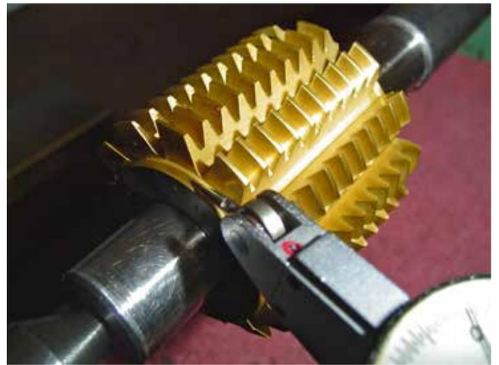
Figure 2: Example of indicating hub radial runout.
