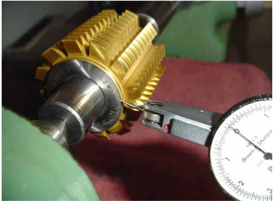
Figure 3: Example of indicating hub face runout.
