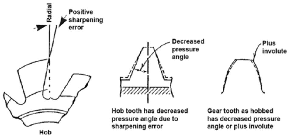
Figure 4: Hob with positive rake error.
