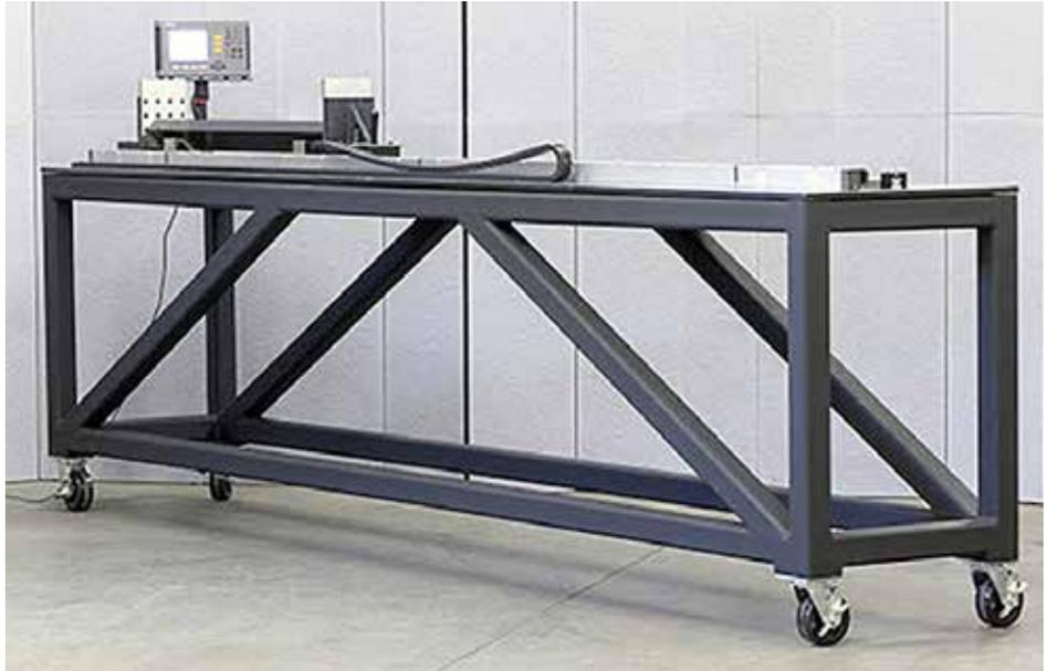
The Barstock Table is designed for checking bar stock materials. (Courtesy: Raytech Measuring Systems)
